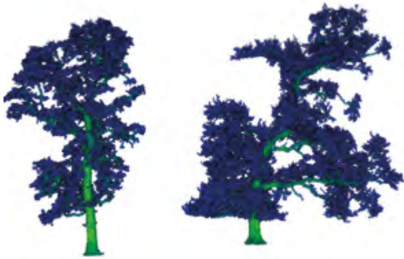
3D point cloud of storm damaged Oak using a ZEB Horizon scanner
