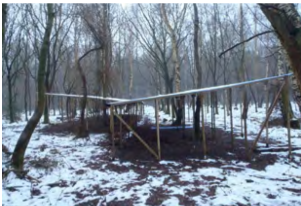
Figure 2: Rain exclusion shelter constructed around stems of Oak trees to simulate drought under experimental conditions
