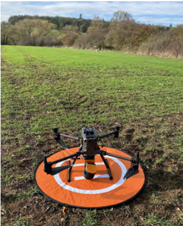
DJI Matrice 300 RTK drone with GeoSLAM LiDAR scanner
